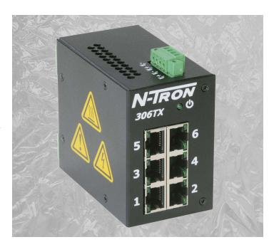
The *N-TRON*<sup>™</sup> 306TX Industrial Network Switch is designed to a climate controlled environment. The 306TX has extended operating environmental specifications to meet the harsh needs of the industrial environment. For cost savings and convenience the network switch can be DIN-RAIL mounted alongside Ethernet I/O or other Industrial Equipment.
