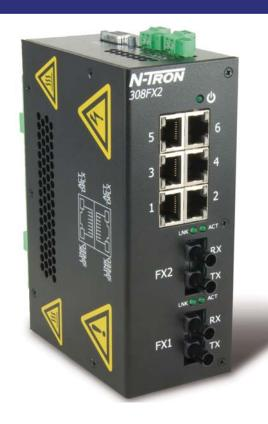
The 308FX2-N simplifies plant wiring by eliminating the need to bring data acquisition and control connections back to a climate controlled environment. The switch has extended operating specifications to meet the harsh needs of the industrial environment, including extended temperature rating, extended shock and vibration specs, redundant power inputs, and a high MTBF (greater than 2M hours).
