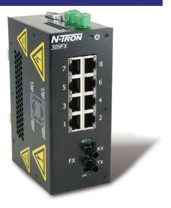
The 309FX-N simplifies plant wiring by eliminating the need to bring data acquisition and control connections back to a climate controlled environment. The switch has extended operating specifications to meet the harsh needs of the industrial environment, including extended temperature rating, extended shock and vibration specs, redundant power inputs, and a high MTBF (greater than 2M hours).
