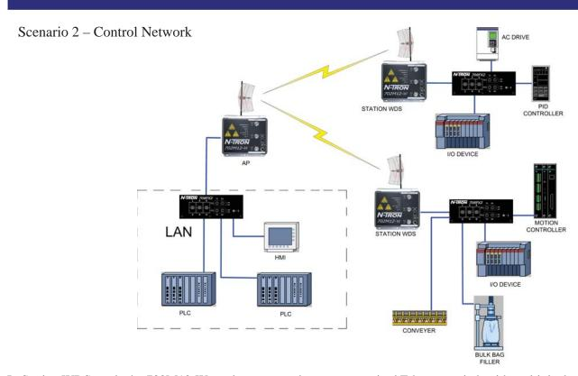
In Station WDS mode the 702M12-W can be connected to a remote wired Ethernet switch with multiple devices connected to the switch.
