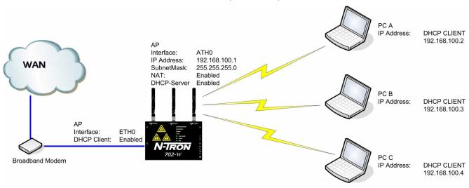
*N-TRON 702-W* confured as a powered Router allows layer 3 routing to set up network segmentation. It supports the Network Address Translation (Masquerading) feature which is widely used by Access Points. NAT will act as the firewall between LAN and WLAN networks. Additional Firewall settings can be configured for Layer 3 packet filtering and access control in Router mode. It can also act as a DHCP server, automating the assigning of IP addresses.
